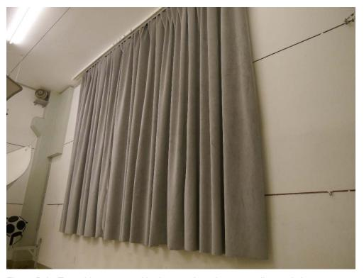
Figure B.2. Test object mounted in the reverberation room, diagonal view.
